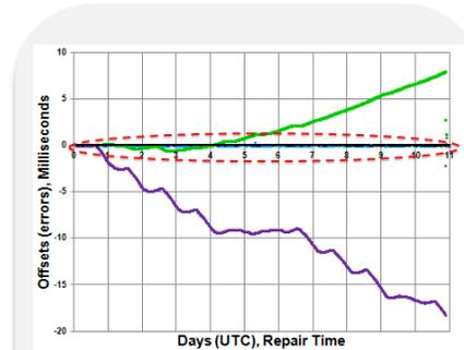
← Zoom-in of circled area above. RB in holdover virtually the same as GPS over test period (+/- 10 microseconds).
